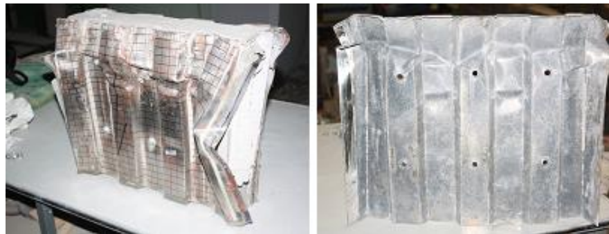
(b) failure mode of specimen with stopping edge
