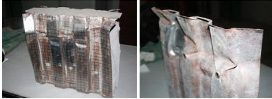
(a) failure mode of panel without stopping edge with outward buckling of steel
