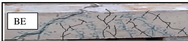
Figure 31. Crack Pattern for beam (BE) after 60 days of Corrosion Acceleration
