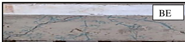
Figure 25. Crack Pattern for beam (BE) after 30 days of Corrosion Acceleration
