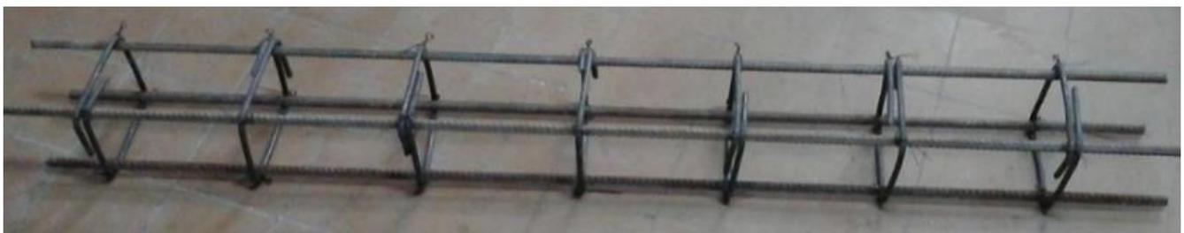
Fig. 2. Upper and lower specimen reinforcement.
