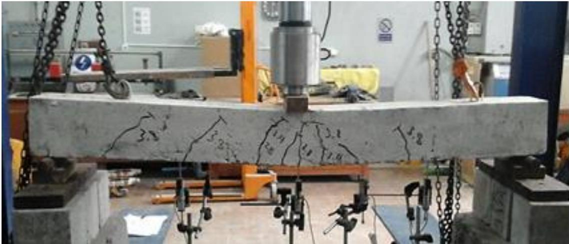
Fig. 6. Reference beam crack pattern.
