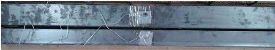
Fig. 5. Mid-span strain gauge.
