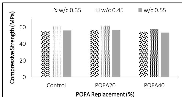
Fig. 2. The effect of water-cement ratio towards compressive strength of POC LWAC with POFA.
