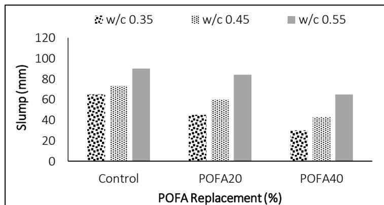
Fig. 1. The effect of water-cement ratio towards workability of POC LWAC with POFA.
