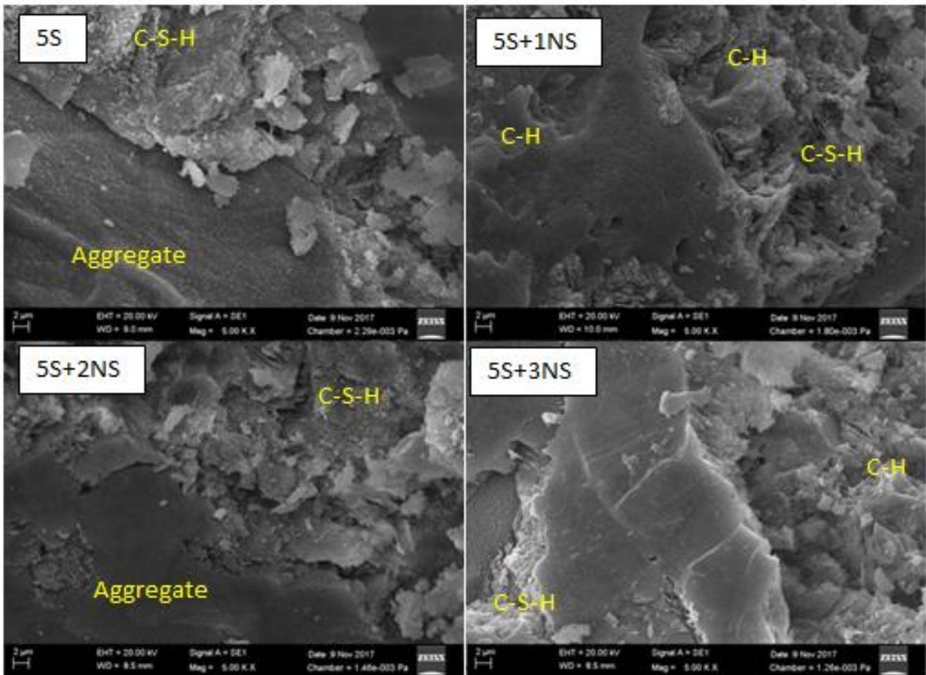
Fig. 7. SEM images of the mortar admixtures.
