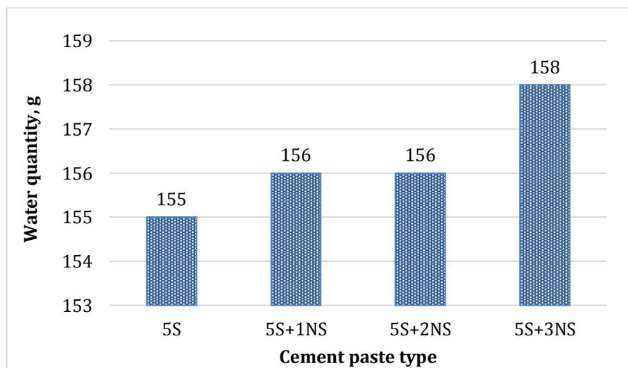
**Fig. 3.** Water necessities of cement pastes with micro and nano silica substitutions.
