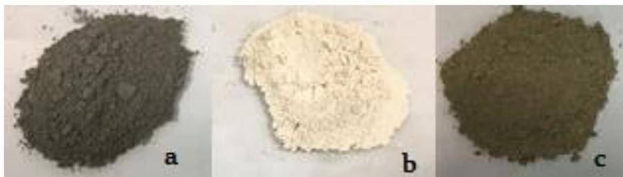
**Fig. 2.** a) Micro silica; b) Nano silica; c) Cement.**Table 3.** Standard sand sieve analysis.
