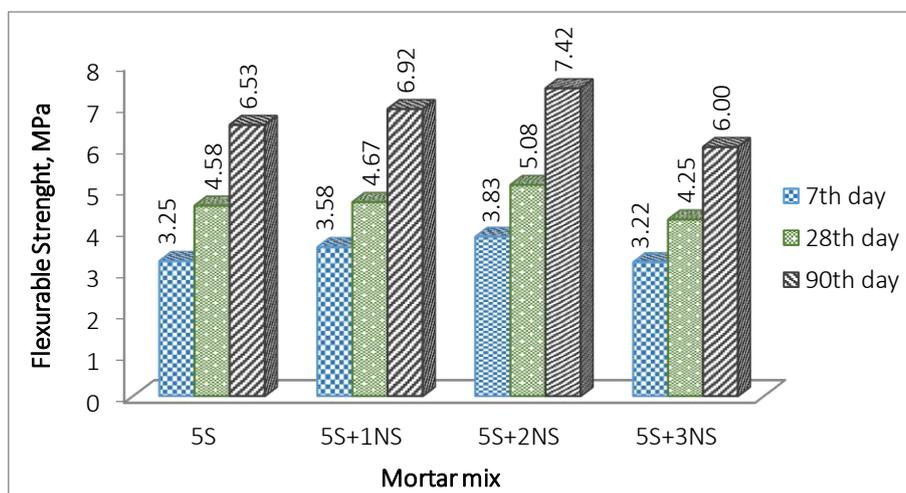
Fig. 5. Flexural strength results of mortar mixtures.
