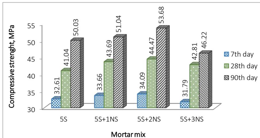
**Fig. 6.** Compressive strength results of mortar mixtures.**Table 7.** According to 5% micro silica added mortars, the effect of nano silica substitution over compressive strength (+, increases; -, decreases).
