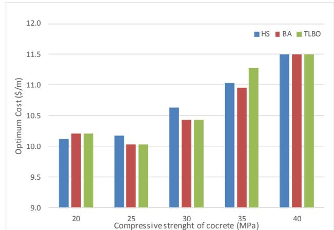
**Fig. 2.** The optimum costs for 250 kNm flexural moment.
