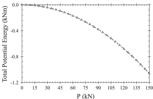
**Fig. 7.** Potential energy value of increasing loading for MAT1 material.
