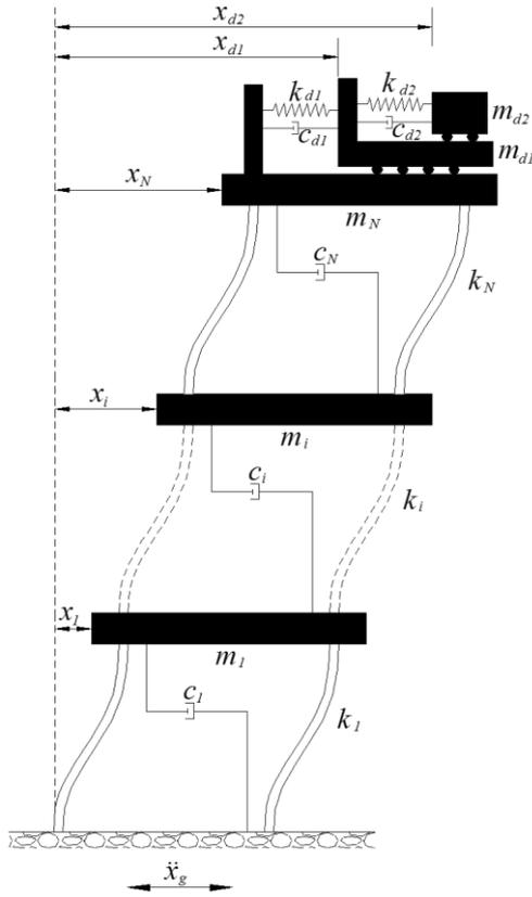
Fig. 1. Model of N-story shear building with a DTMD.
