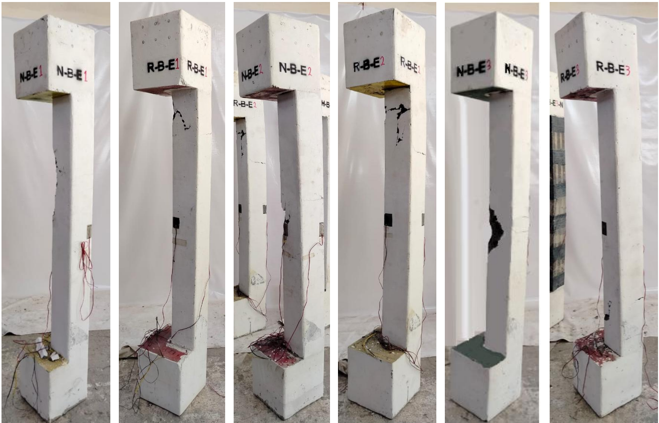
Fig. 16. Observed failure modes of the tested specimens.
