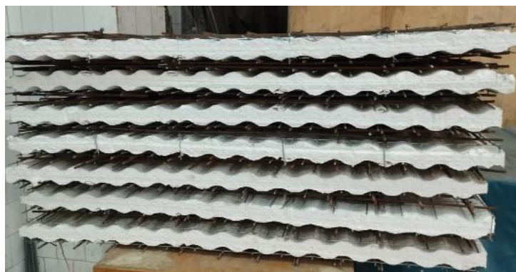
Fig. 10. Corrugated foam panels used.
