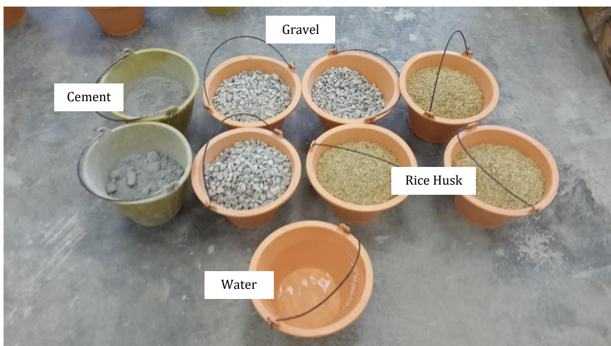
Fig. 2. The basic ingredient of pervious concrete with RH.
