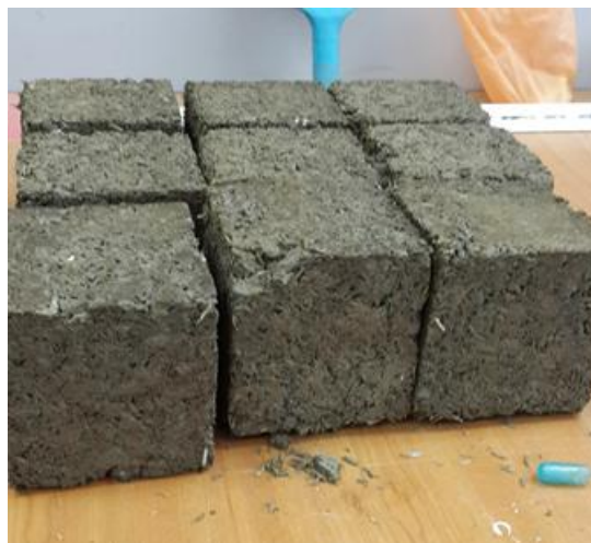
Fig. 5. The cube specimen with 8% of RH in pervious concrete.
