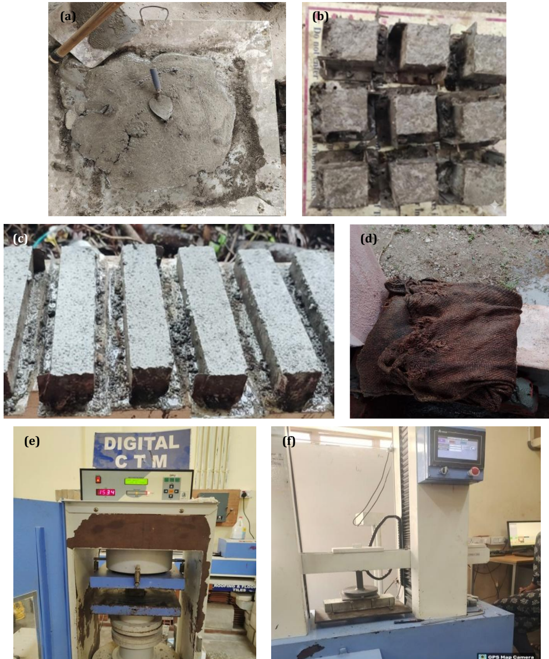
Fig. 1. Experimental program illustrating: (a) ECC mixing and specimen preparation; (b) Casting of cube; (c) Beam specimens; (d) Curing of specimen; (e) Compressive strength testing setup; (f) Bending test setup.
