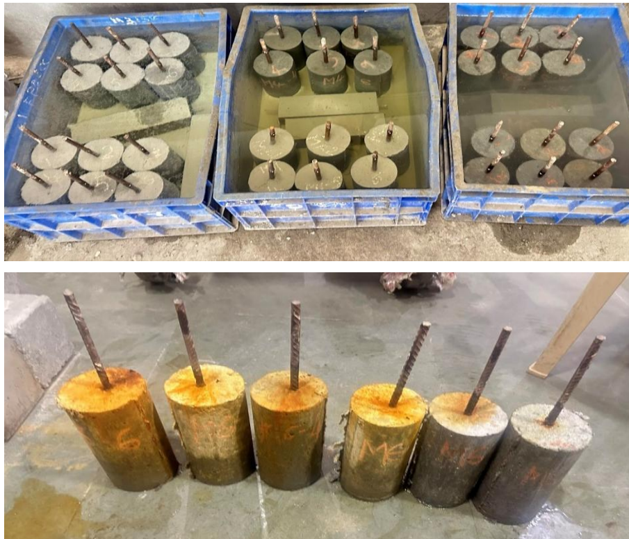
Fig. 5. Specimens used for accelerated corrosion testing during curing and after corrosion.
