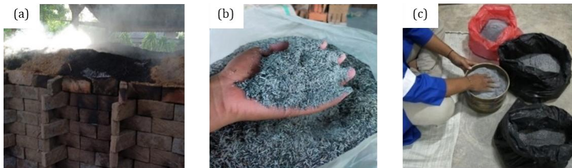
Fig. 2. Production process of rice husk ash (RHA): (a) Red brick firing process; (b) Produced RHA; (c) Sieving of RHA.
