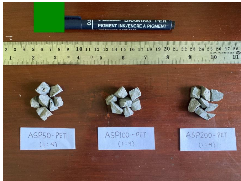
Fig. 5. Manufacturing results and material testing of artificial coarse aggregate.
