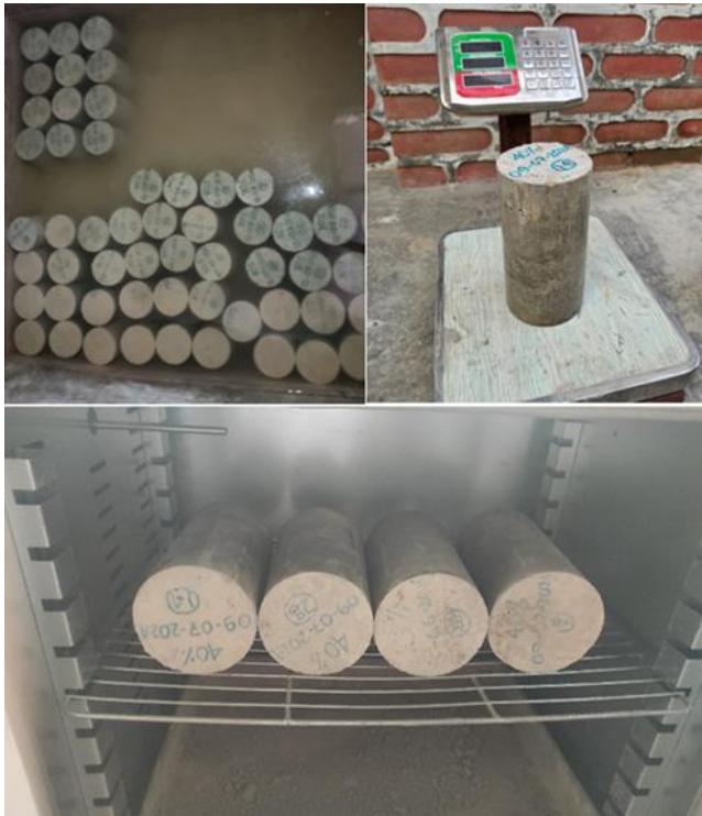
Fig. 4. Water absorption capacity test conducted in this study.
