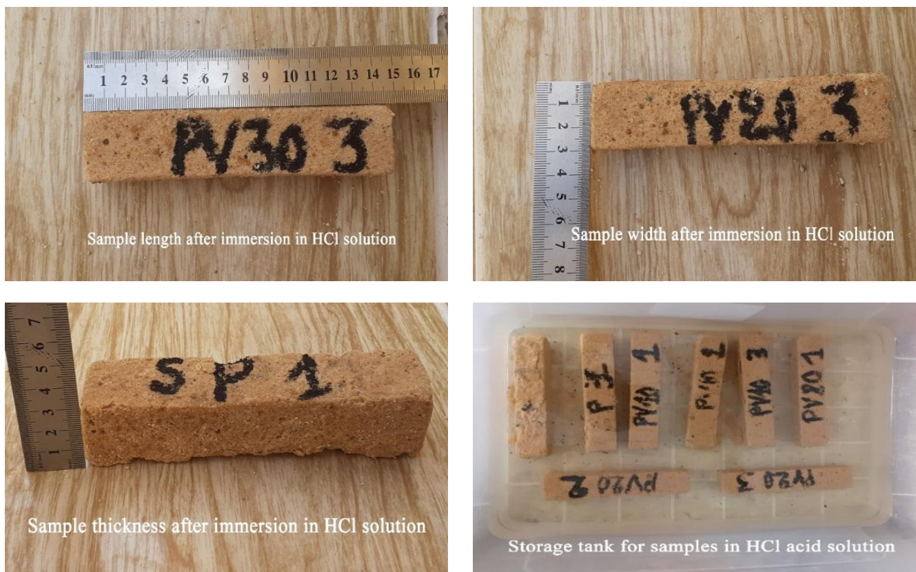
Fig. 13. Visual examination of concretes exposed to acid solution at 90 days.
