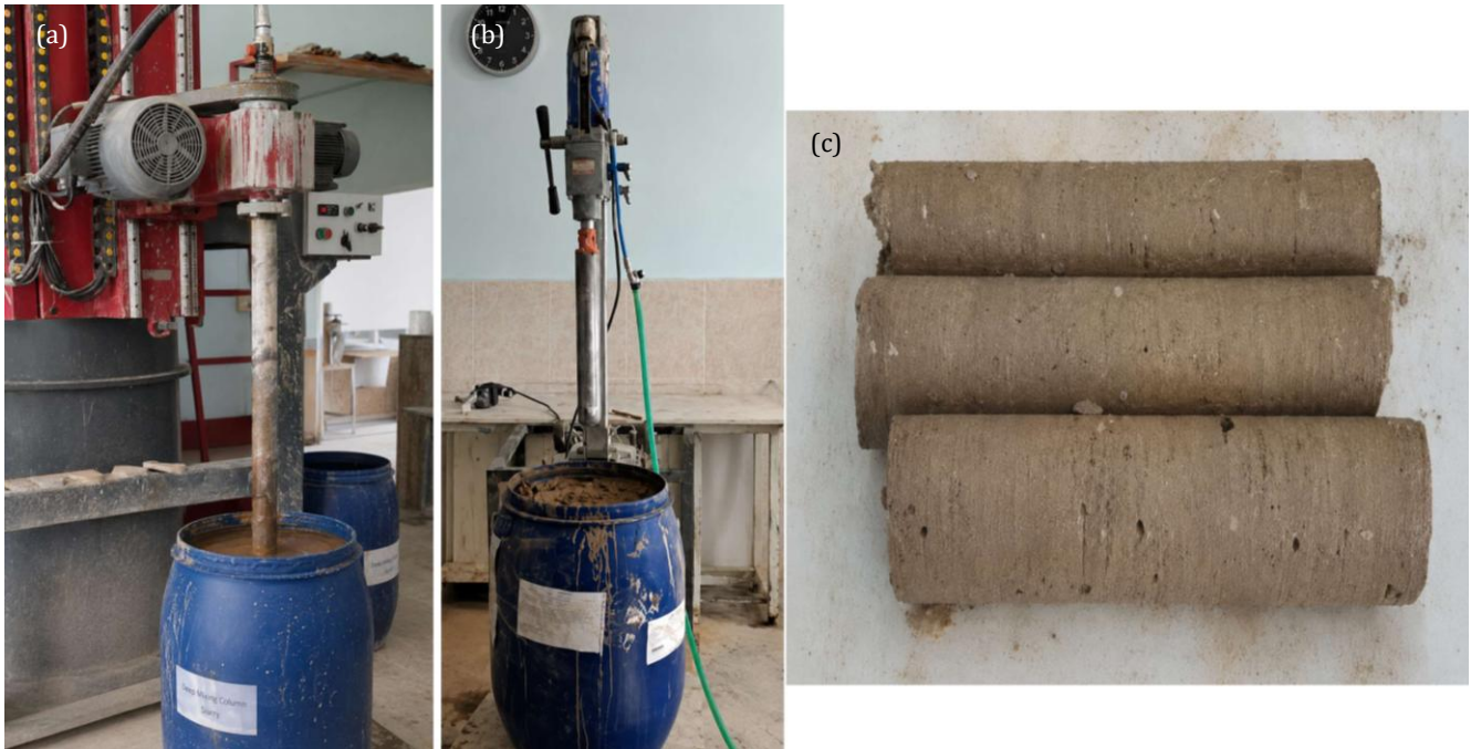
Fig. 2. DSM column formation and core sampling: (a) DSM column formation in preparation container; (b) Core sampling; (c) Core samples.
