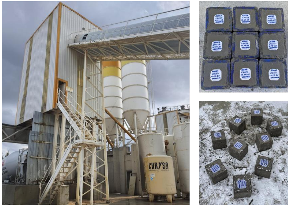
Fig. 2. Production of concrete samples in a ready-mix concrete plant.
