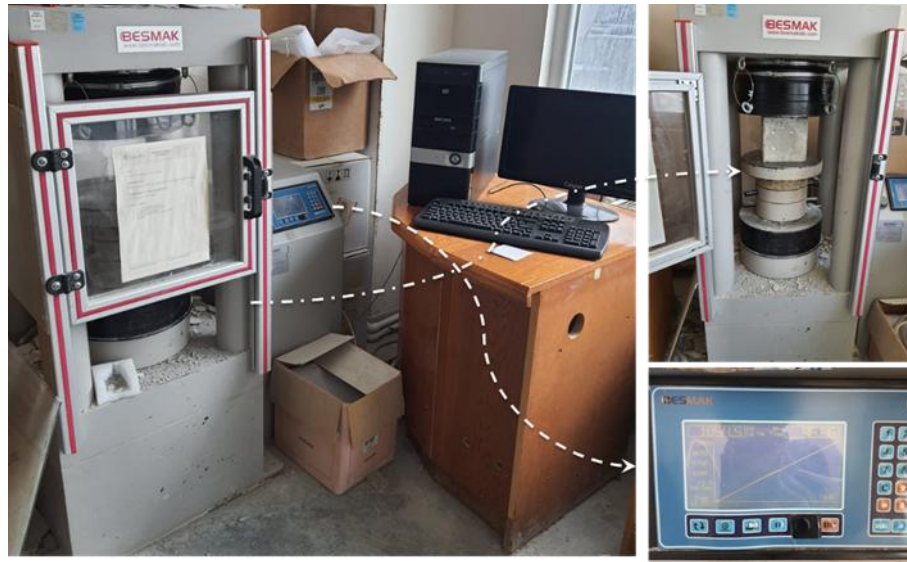
Fig. 4. The photograph of the compressive strength testing press.
