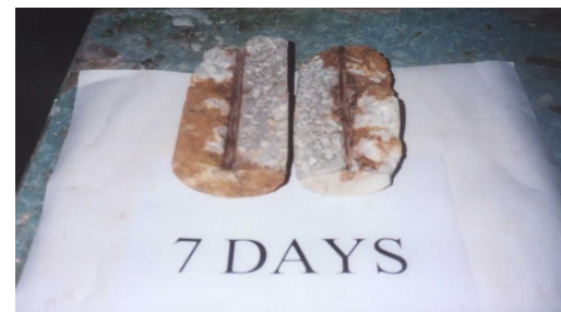
Fig. 19: Modes of Failure in SCC2 Cylinders after 2, 4 and 7 days of Exposure to (MgSO_4) .
