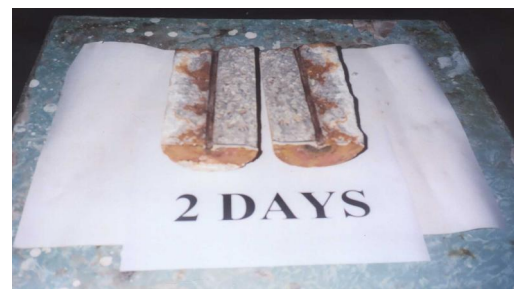
Fig. (18): Modes of Failure in NC Cylinders after 2, 4 and 7 days of Exposure to (MgSO_4) .
