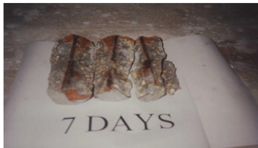
Fig. (18): Modes of Failure in NC Cylinders after 2, 4 and 7 days of Exposure to (MgSO_4) .
