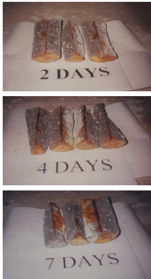
Fig. 20: Modes of Failure in SCC3 Cylinders after 2, 4 and 7 days of Exposure to (MgSO 4 ).
