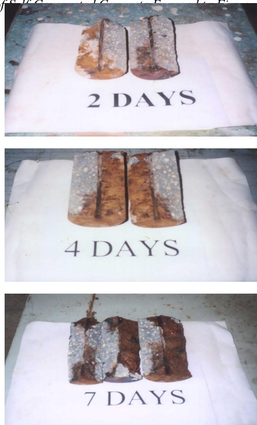
Fig. 22: Modes of Failure of SCC2 Cylinders after 2, 4 and 7 days of exposure to (MgCl 2 )
