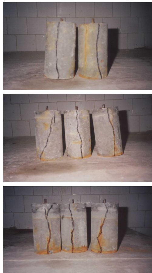
Fig. 21: Modes of Failure in SCC1 Cylinders after 2, 4 and 7 days of Exposure to (MgCl 2 ).
