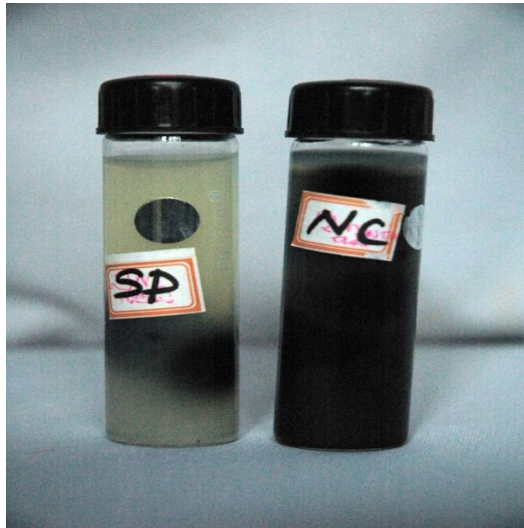
Fig 4: Growth of SRB indicated in Modified Postgate medium by blackening showing density of SRB higher on normal concrete MIX-I biofilm compared to admixture concrete MIX-2 biofilm
