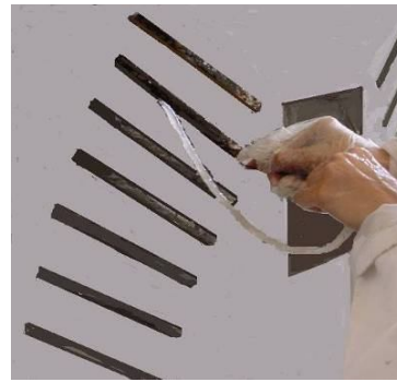
Fig. 5: NSM intertwined rods were stitched through the beam
