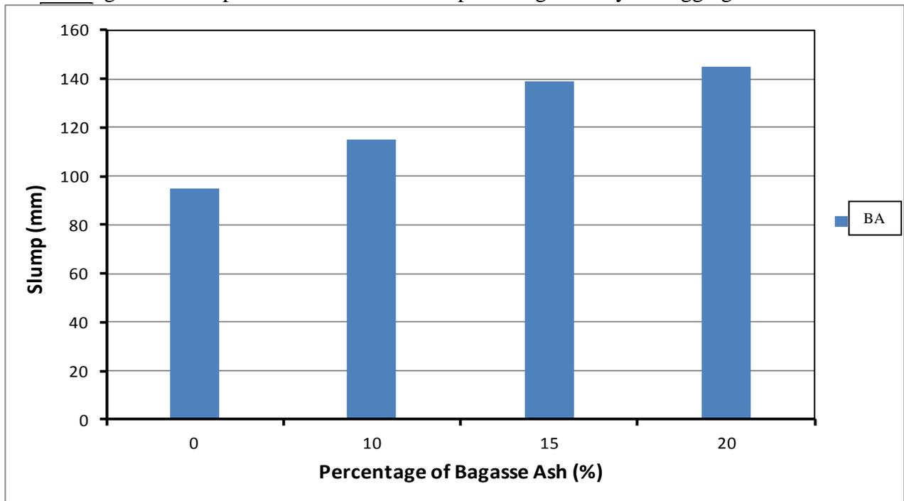
Figure 2: Slump test values for different percentage of bagasse ash.
