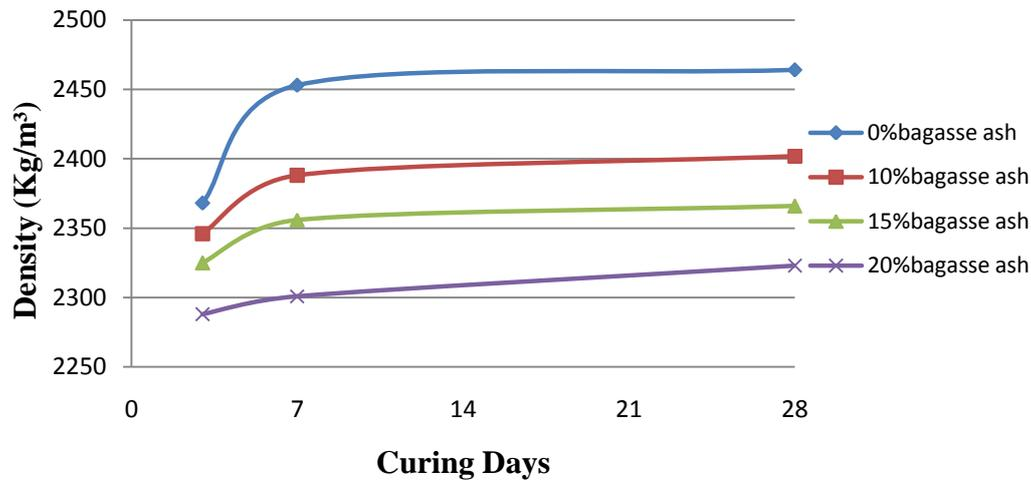
Figure 10: Average bagasse ash density vs. curing days
