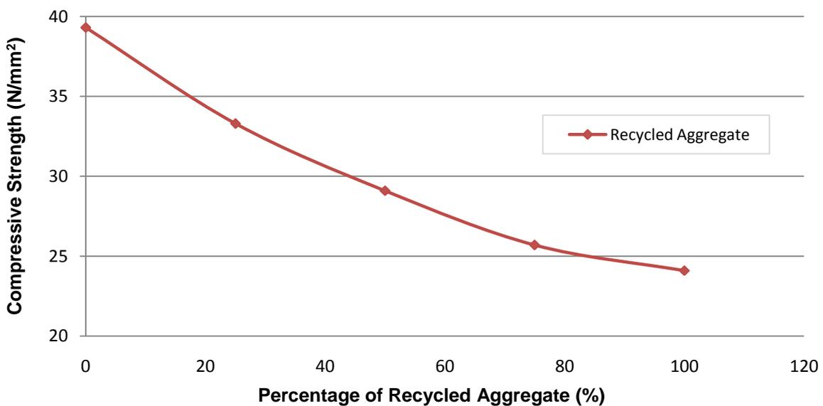
Figure 7: Average recycled aggregate compressive strength vs. percentage of recycled aggregate
