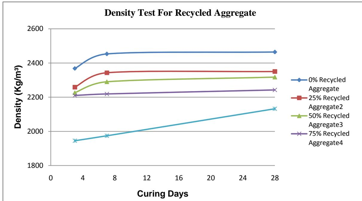
Figure 9: Average recycled glass density vs. curing days
