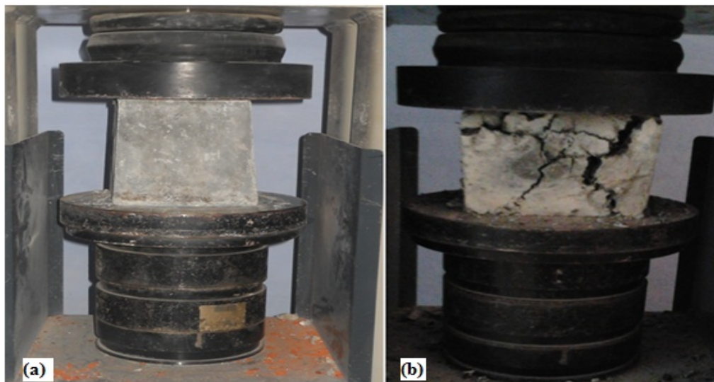
Figure 2: Cube specimen under compression testing before (a) failure (b) after failure.
