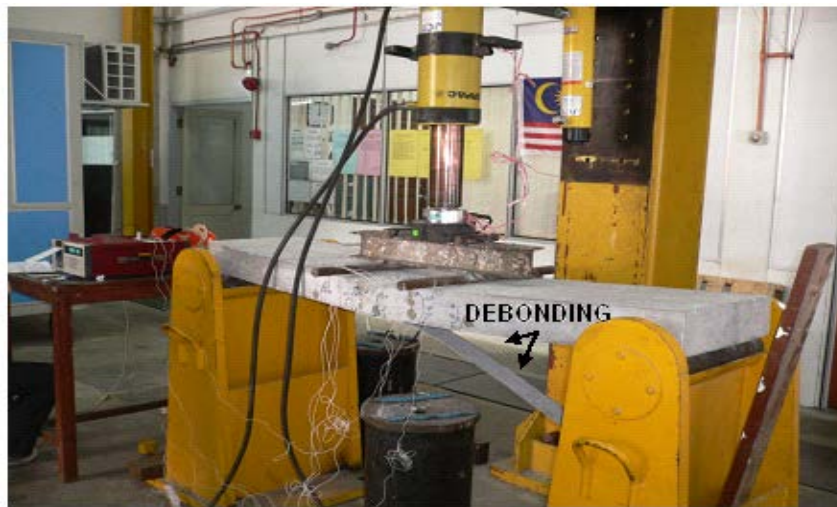
Figure 5: CFRP debonding at the CFRP/concrete interface under line load.
