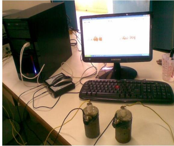
Figure 2. Laboratory set up for AE measurement
