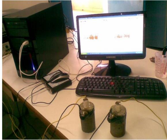
Figure 2. Laboratory set up for AE measurement
