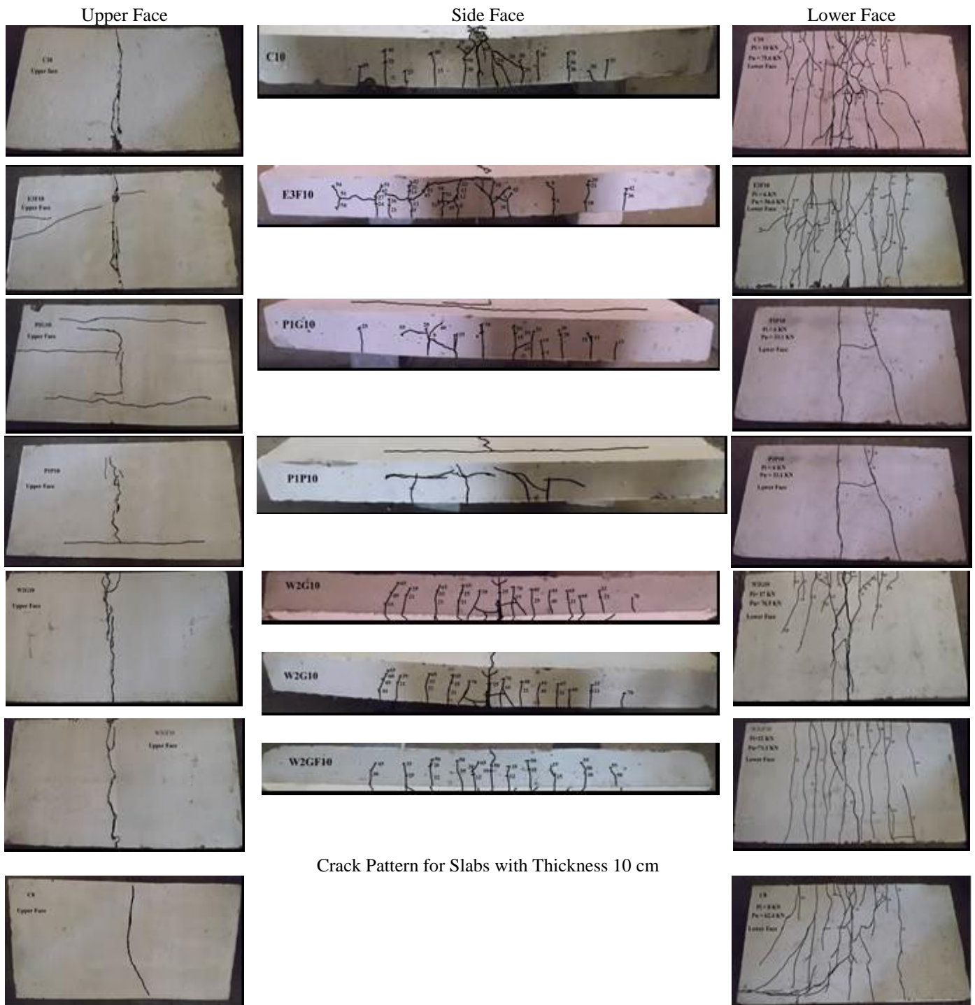
Figure 40: Crack Pattern for Slabs with Thickness 10 cm.
