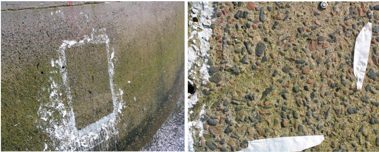
Figure 7. Area of ice shield pier used to create silicon mould; normal view (left), close-up view (right); (the white residues borders the area where the mould was cast) [31].
