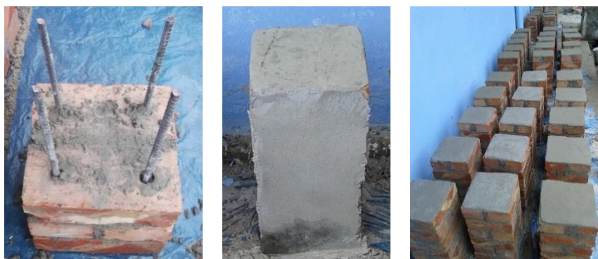
Fig. 2. Photos of constructing specimens for testing.
