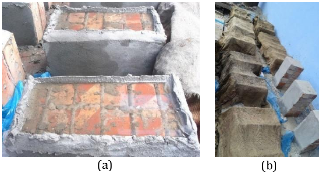
Fig. 3. Applying 10% NaCl solution into specimens: (a) NaCl solution on top surface; (b) Covering the specimens (for curing).
