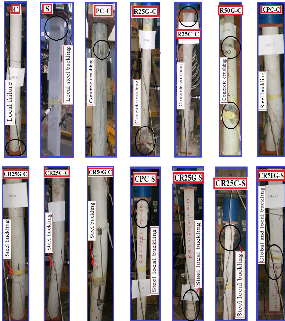
Fig. 11. Failure mode of tested specimens.
