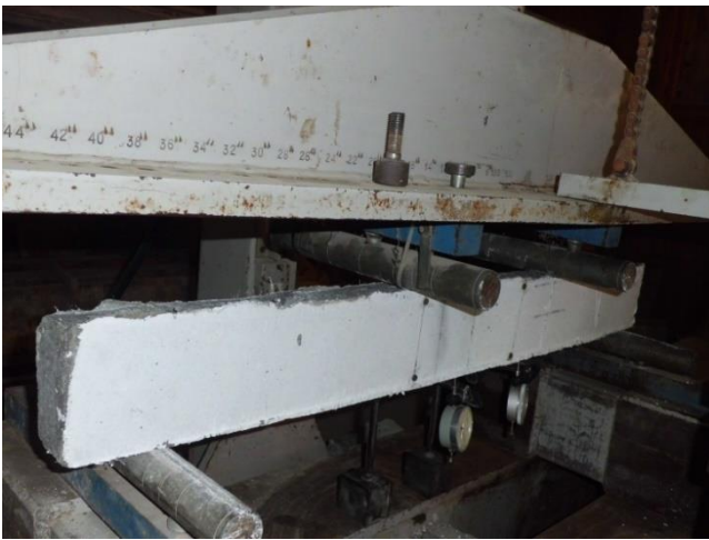
Fig. 18. ELE flexural 100KN testing machine.
