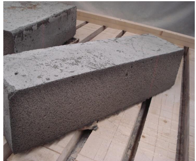
Fig. 3. Lightweight concrete sample.
