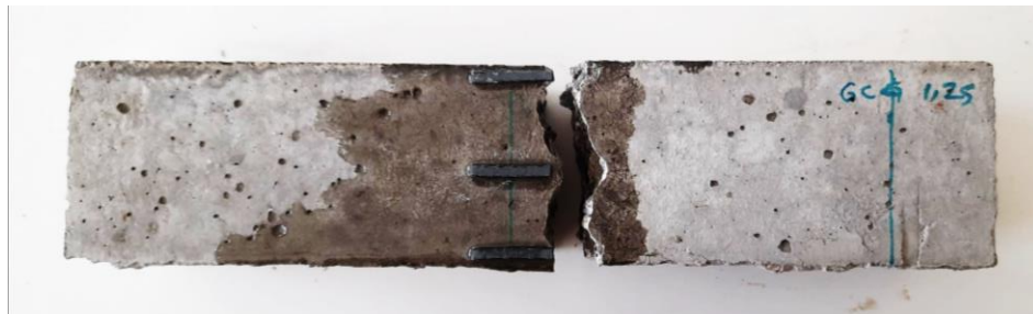
Fig. 5. Fracture mode of concrete reinforced with laminate pieces.
