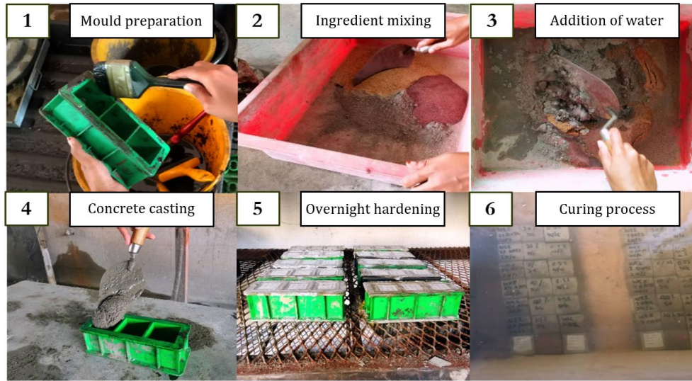
Fig. 6. Mortar specimen preparation process.
