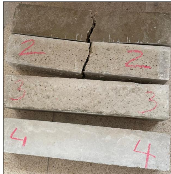
Fig. 3. Damaged and undamaged concrete specimens.
