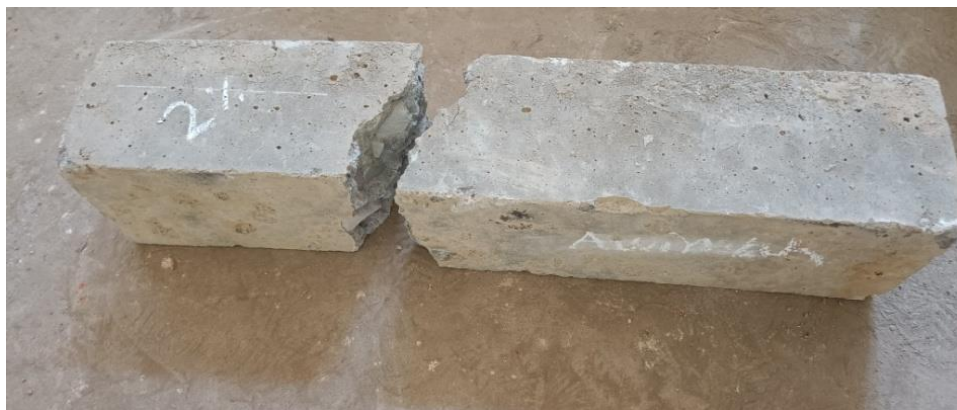
Fig. 8. Beam specimen after the flexural strength test.
