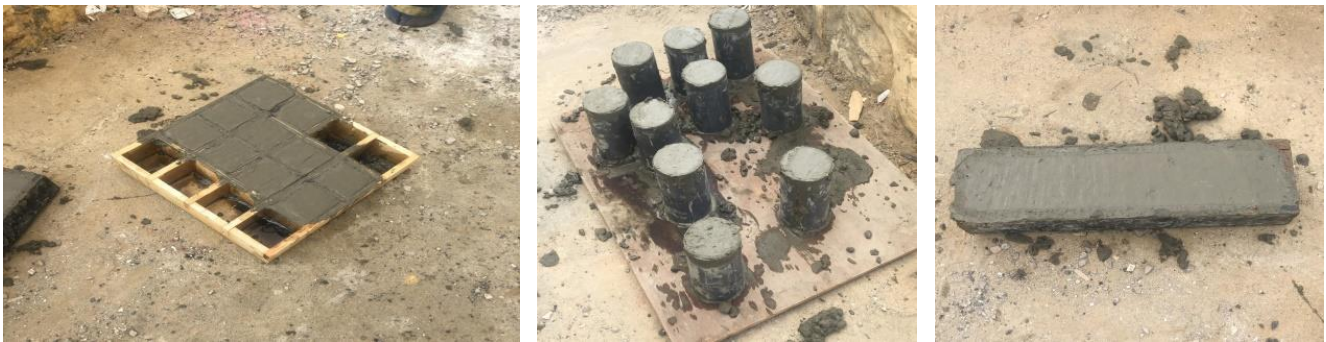
Fig. 3. Shapes of test molds: cubes, cylinders, and beams.
