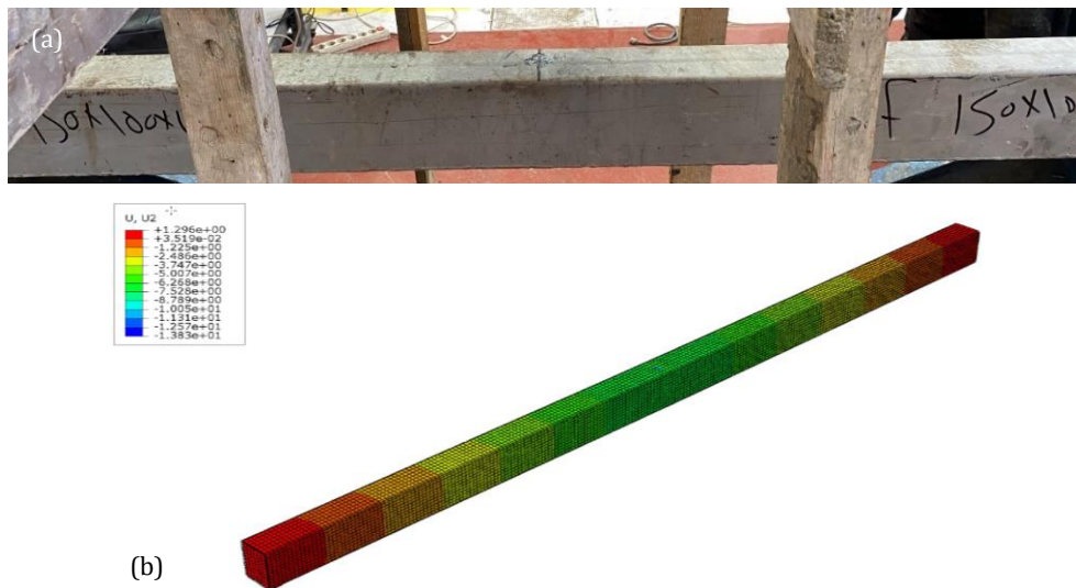
Fig. 13. Deformed shape of 100X150X4 filled single-cell column (SCC-F): (a) Deformed shape of tested specimen; (b) Deformed shape of tested specimen's FE model.
