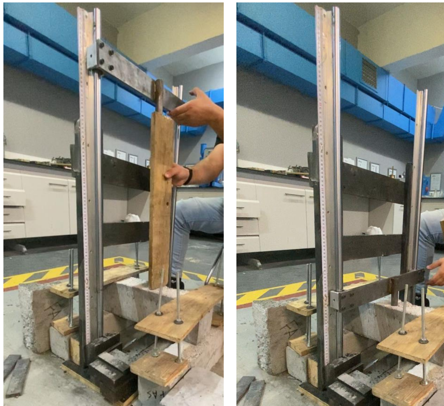
Fig. 5. Impact test of concrete.
