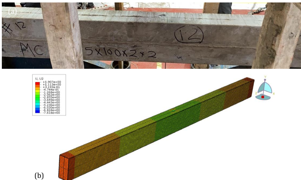
Fig. 20. Deformed shape of 100X225X2X2 filled multi-cell column (MCC-F): (a) Deformed shape of tested specimen; (b) Deformed shape of tested specimen's FE model.
