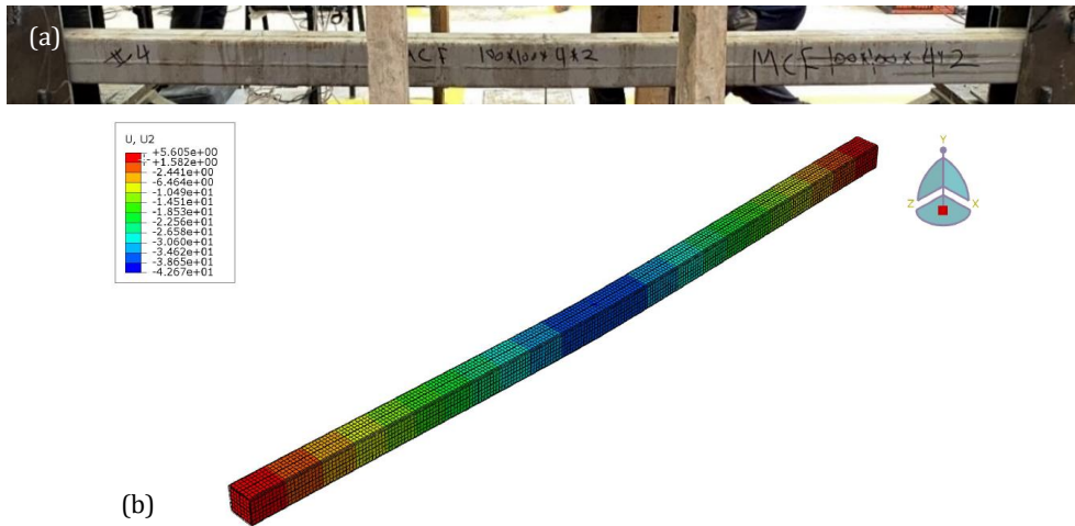
Fig. 18. Deformed shape of 100X100X4X2 filled multi-cell column (MCC-F): (a) Deformed shape of tested specimen; (b) Deformed shape of tested specimen's FE model.
