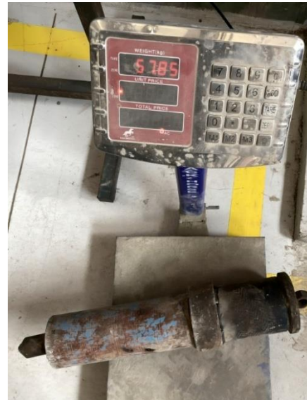
Fig. 1. Details of drop weight (impactor) (all dimensions are in mm).
