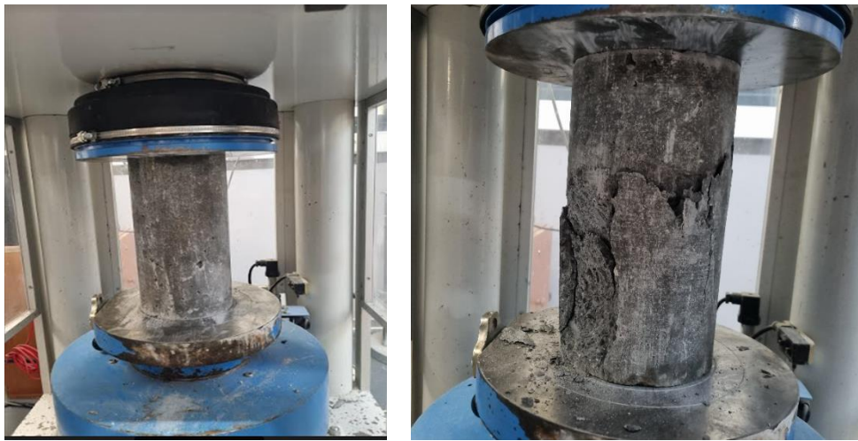
Fig. 4. Compressive strength test of concrete.
