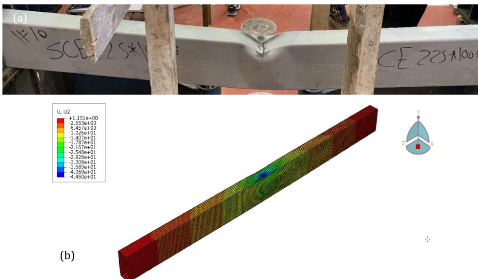
Fig. 11. Deformed shape of 100X225X3 empty single-cell column (SCC-E): (a) Deformed shape of tested specimen; (b) Deformed shape of tested specimen's FE model.
