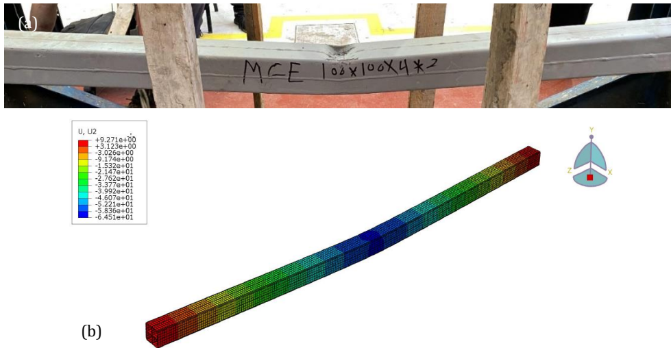
Fig. 15. Deformed shape of 100X100X4X2 empty multi-cell column (MCC-E): (a) Deformed shape of tested specimen; (b) Deformed shape of tested specimen's FE model.
