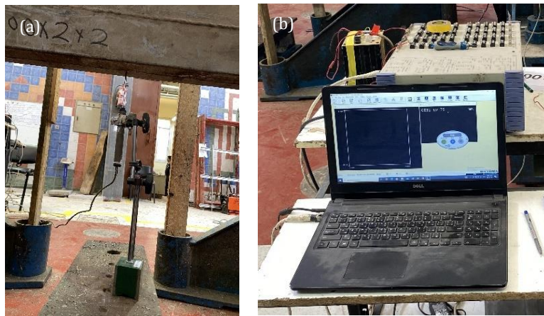
Fig. 3. Displacement with time measurement device: (a) LVDT device; (b) Data logger and computer.
