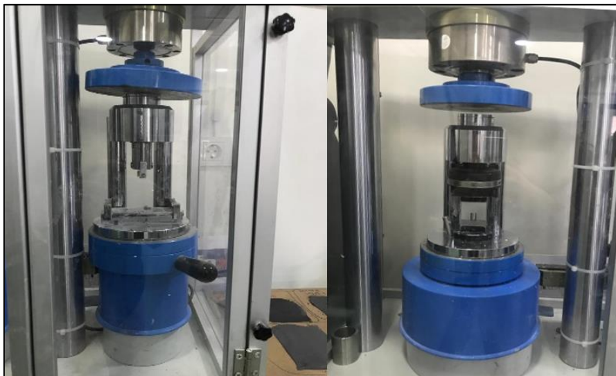
Fig. 9. Flexural and compressive strength test setup.
