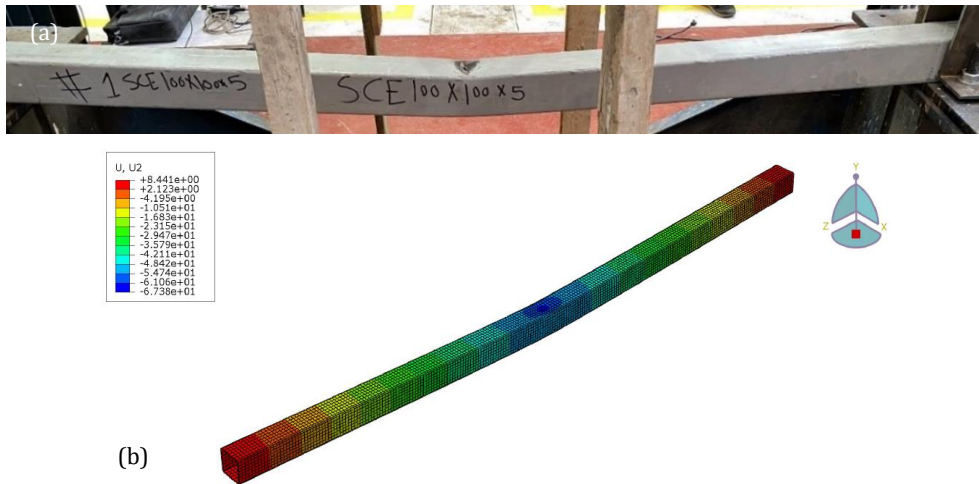
Fig. 9. Deformed shape of 100X100X5 empty single-cell column (SCC-E): (a) Deformed shape of tested specimen; (b) Deformed shape of tested specimen's FE model.
