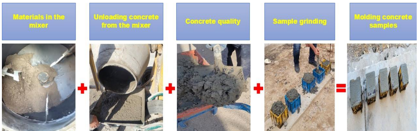
Fig. 4. Heavyweight concrete fabrication stages.
