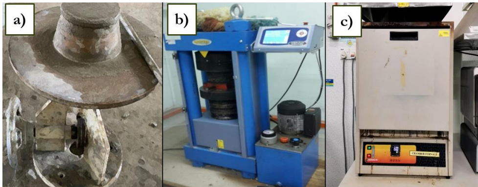
Fig. 7. Testing apparatus used: (a) Flow table; (b) Compression machine; (c) Electric furnace.
