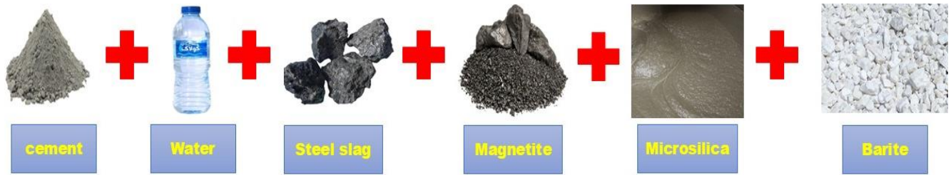
Fig. 3. Components of heavyweight concrete.
