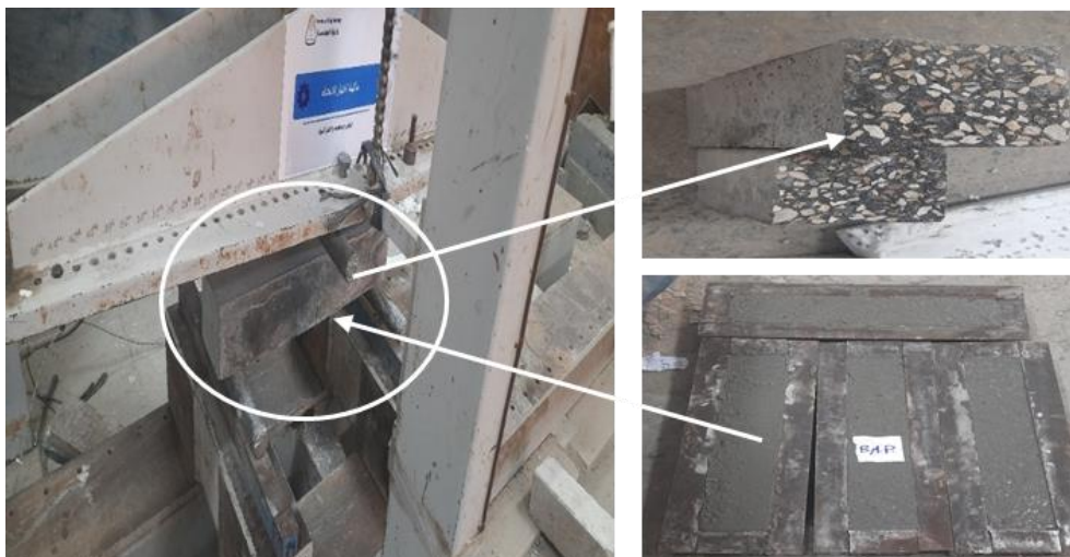
Fig. 8. Flexural strength samples and test setup using a three-point loading system.
