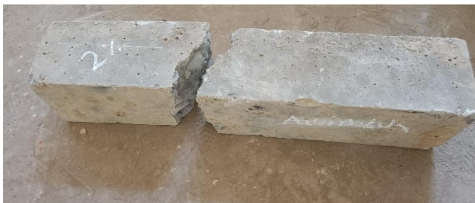
Fig. 8. Beam specimen after the flexural strength test.
