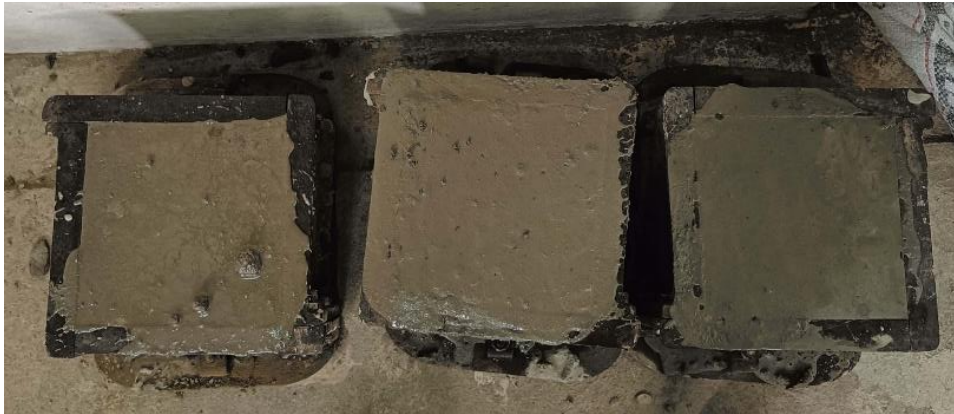
Fig. 2. Fresh concrete cube samples.
