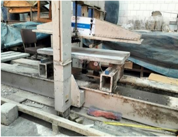
Fig. 12. Four-point loading test setup for slab samples.
