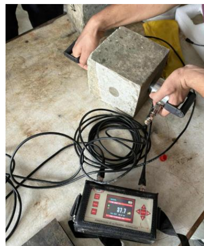
Fig. 6. Ultrasonic pulse velocity test on a concrete cube using the direct method.
