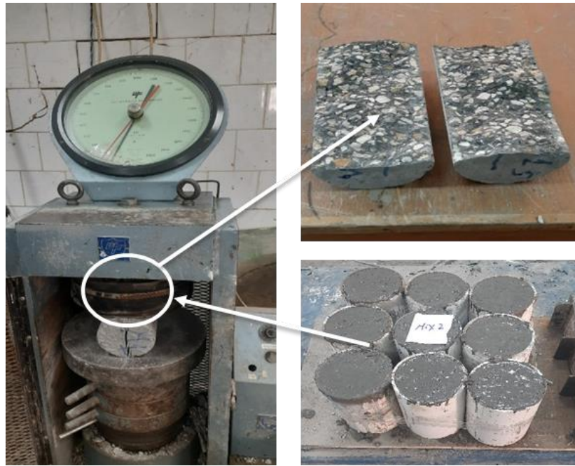
Fig. 10. Splitting tensile strength molds and test setup.
