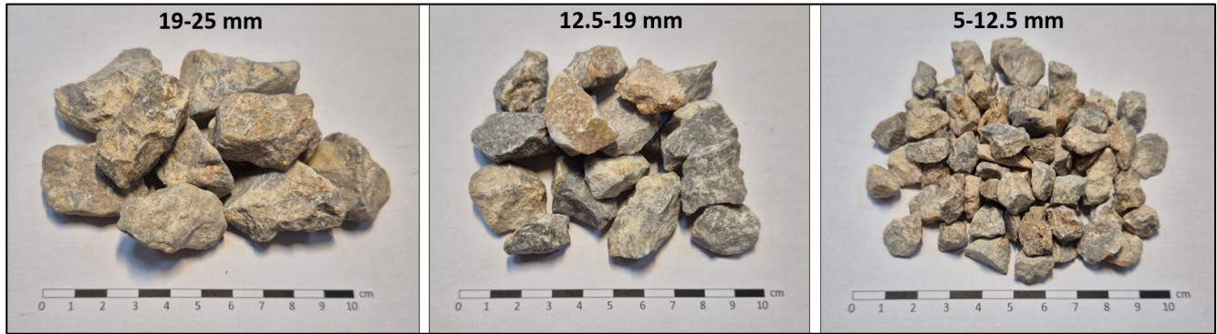
Fig. 1. Coarse aggregates used in RCC mixtures.
