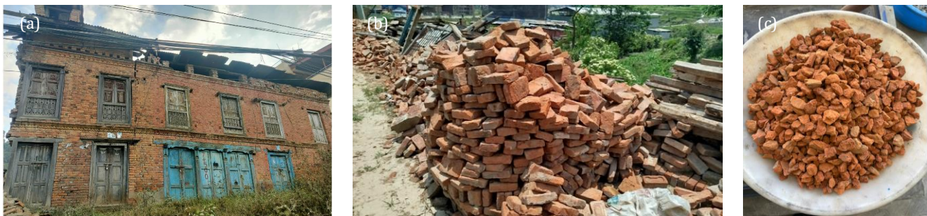
Fig. 3. Collection of bricks and brick aggregates: (a) Century-old brick masonry building located at Sangha, Kabhrepalan-chok, Nepal; (b) Dismantled brick from masonry building; (c) Crushed brick aggregates prepared in laboratory.
