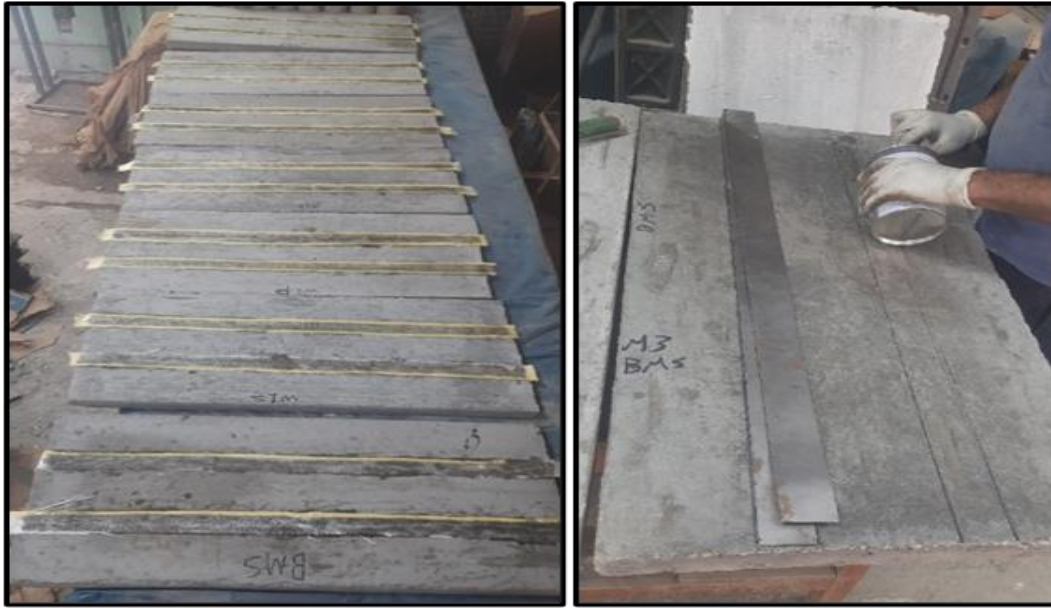
Fig. 4. Glass fiber laminates and steel plate as external reinforcement.
