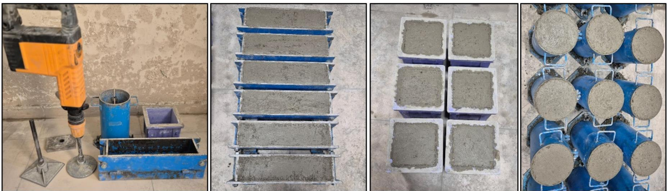
Fig. 4. Vibrating hammer, tamping plates, molds and produced RCC samples.
