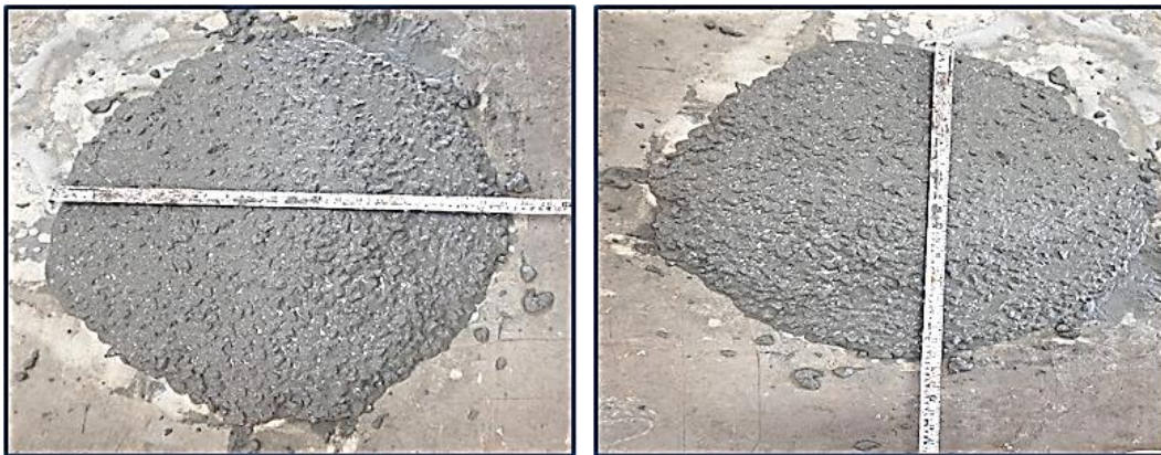
Fig. 5. Flowability of fibrous bio-concrete.
