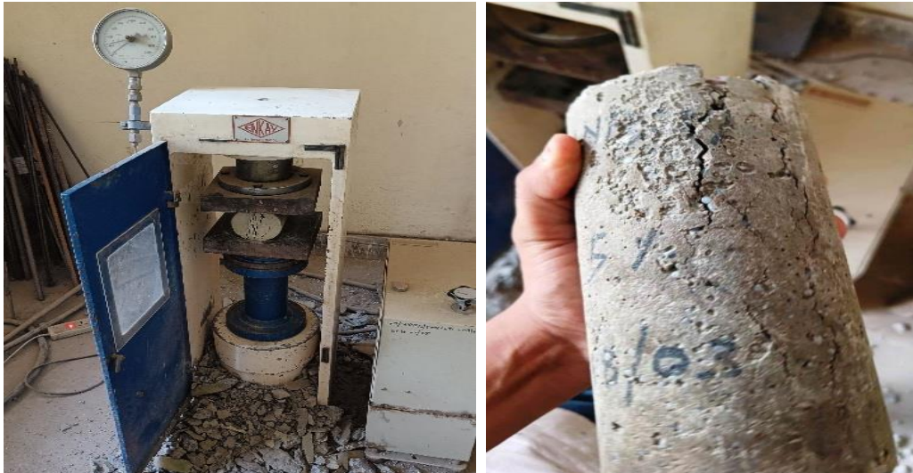
Fig. 6. Splitting tensile strength test of cylindrical specimens.
