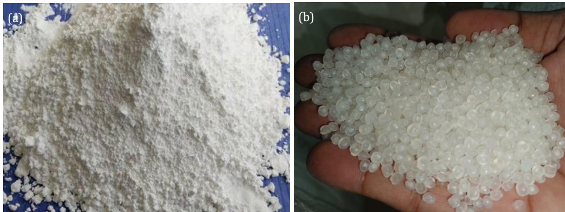
Fig. 1. (a) Nano-CaCO 3 ; (b) PET granules.
