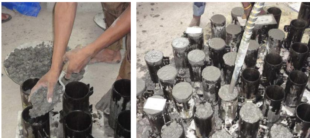
Fig. 1. Specimen preparation and vibration.
