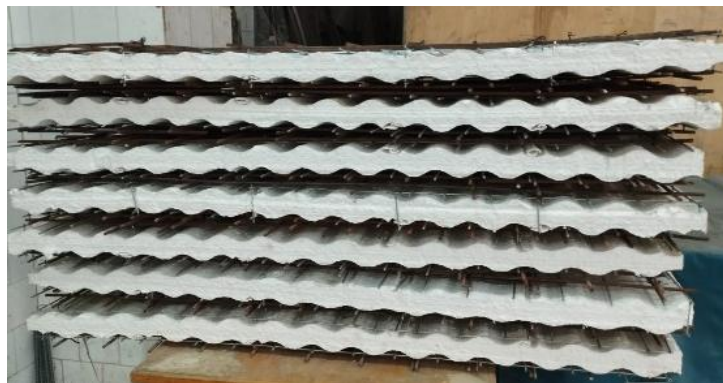
Fig. 10. Corrugated foam panels used.
