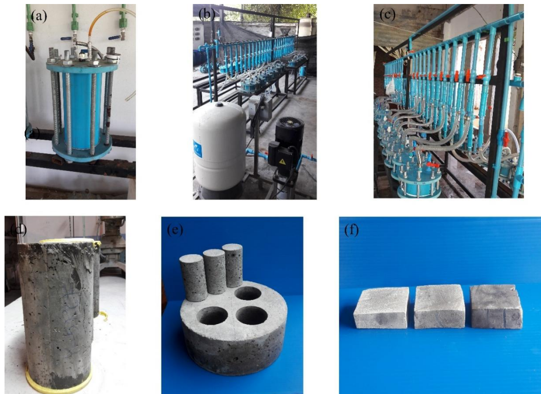
Fig. 2. Experimental setup and representative specimens after calcium leaching: (a) Test cell; (b) Percolation apparatus; (c) Leaching process; (d) RCC specimen; (e) Mortar specimen; (f) Sliced paste samples.
