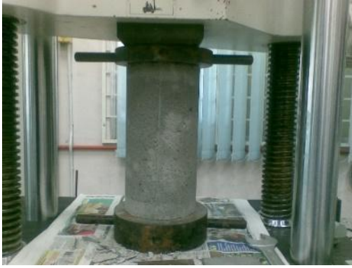
Fig. 2. Failure pattern of concrete cylinder specimen under compressive strength testing.
