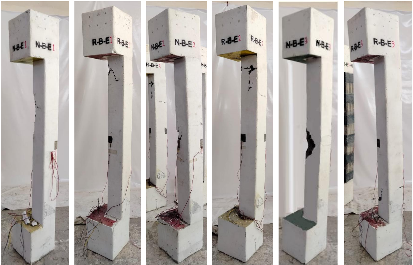
Fig. 16. Observed failure modes of the tested specimens.
