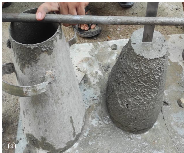
Fig. 5. (a) Workability measurement; (b) Variation of the slump value of the concrete.
