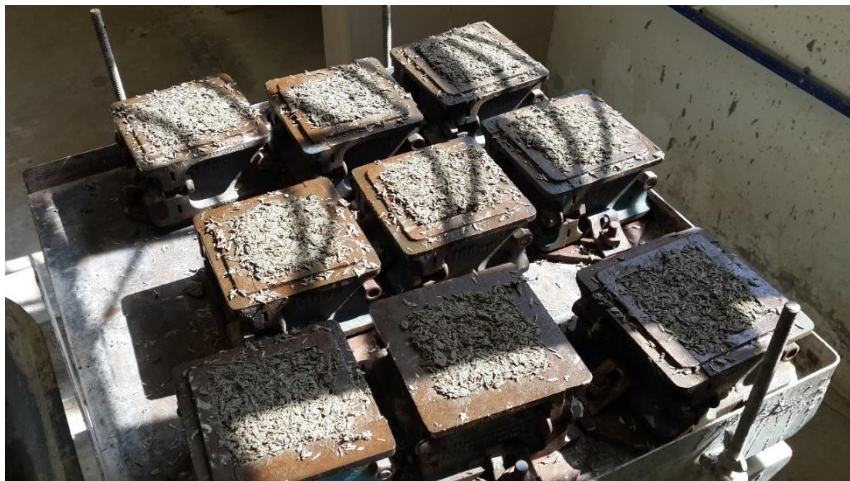
Fig. 4. The process of moulding of pervious concrete on the vibrator table.
