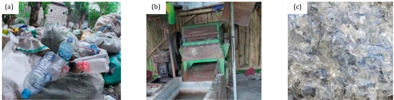
Fig. 1. Treatment process of waste PET plastic: (a) Raw waste PET plastic; (b) Cutting process of PET plastic; (c) Processed PET plastic after cutting.
