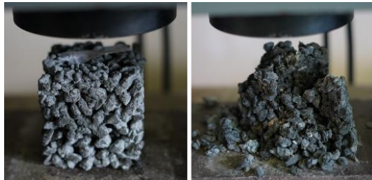
(a) Compression test
