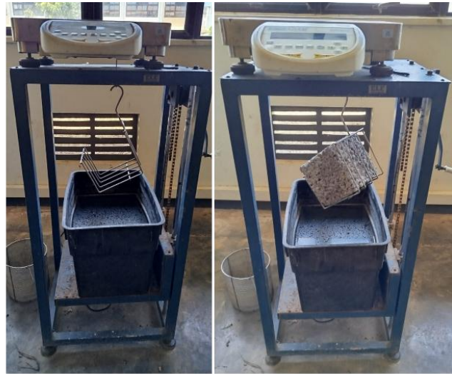
(c) Porosity test
