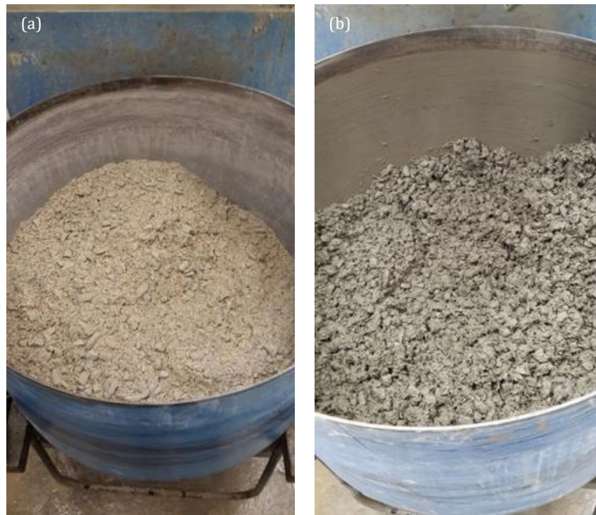
Fig. 3. Pervious concrete mixing: (a) Before adding water; (b) Completing the mixing process.
