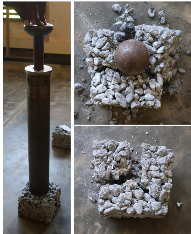
(e) Impact resistance test
