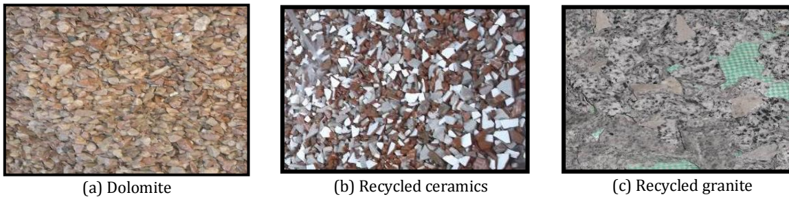
Fig. 2. Natural and recycled coarse aggregates.
