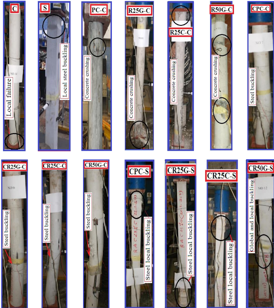
Fig. 11. Failure mode of tested specimens.
