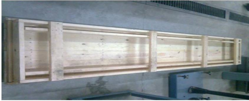
Fig. 4. U shape wooden mold.
