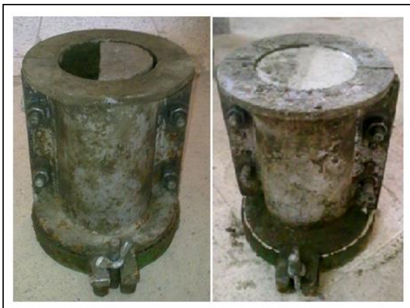
Fig. 3. Composite specimen for splitting tensile strength.
