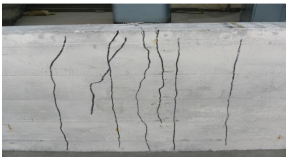
Fig. 26. Crack patterns of all tested slabs.
