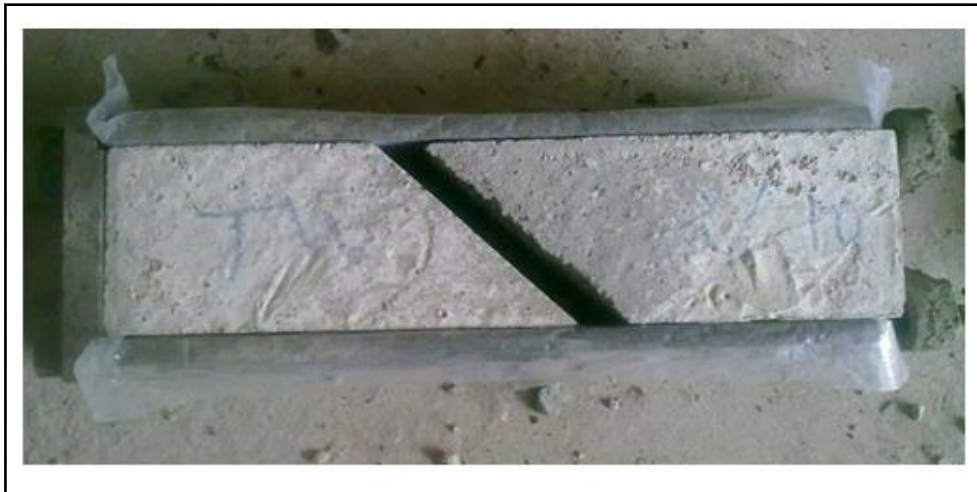
Fig. 6. Composite prism of substrates concrete.
