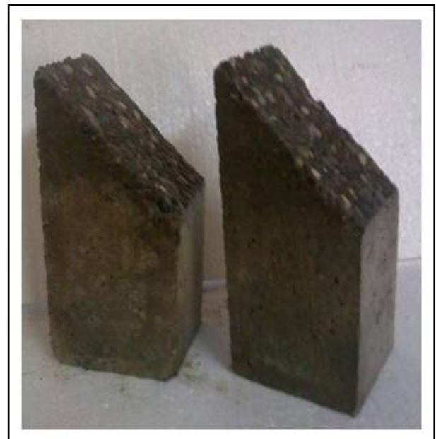
Fig. 5. Sandblast the two halves of NC substrate.
