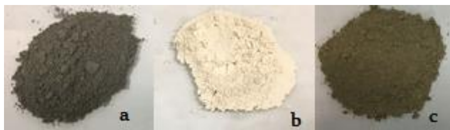
Fig. 2. a) Micro silica; b) Nano silica; c) Cement.
