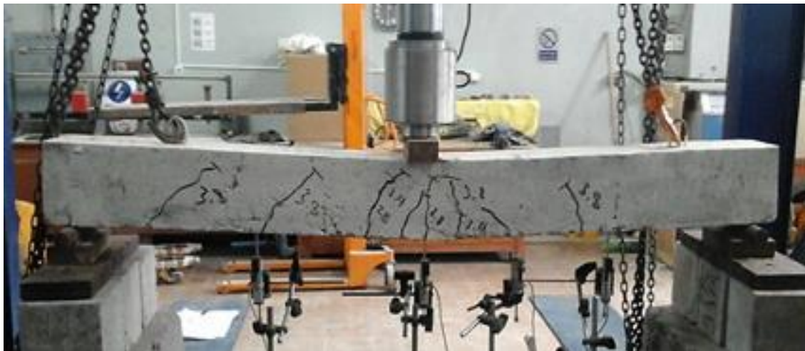
Fig. 6. Reference beam crack pattern.
