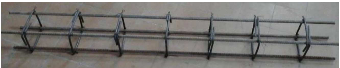
Fig. 2. Upper and lower specimen reinforcement.
