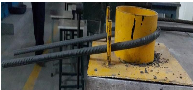
Fig. 10. Coating flexibility test in progress.
