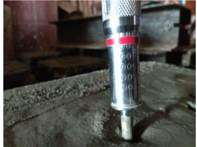
Fig. 2. Penetration resistance test proceeding.
