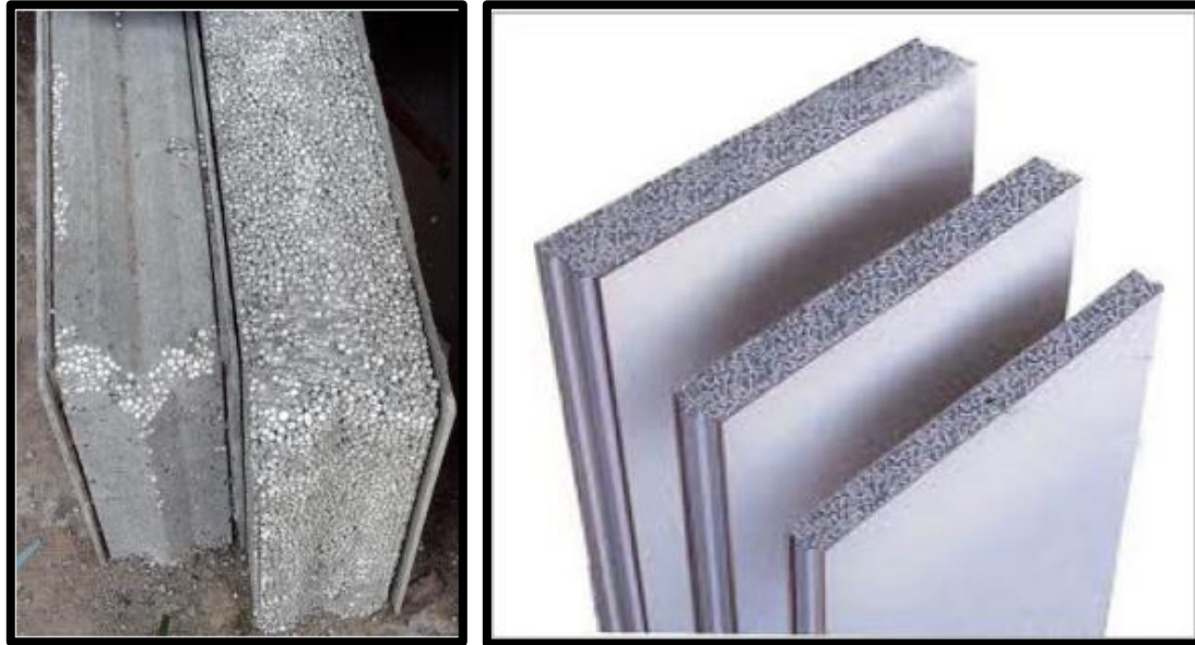
Fig. 1. EPS beads and foam concrete application (Fernando 2015; Dissanayake et al. 2017).
