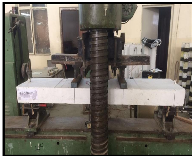
Fig. 4. Preparation of testing slab specimen.
