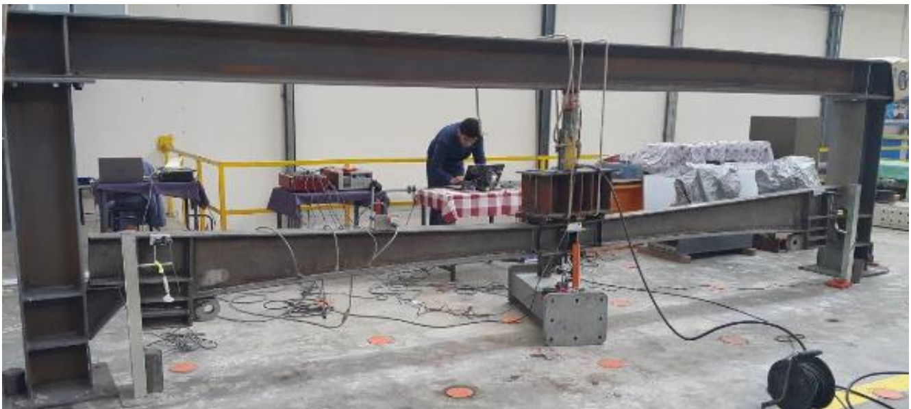
Fig. 27. Test-5 beam (without a cable) after failure.
