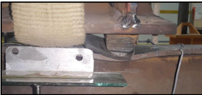
Fig. 19. Buckling of a beam compression flange.
