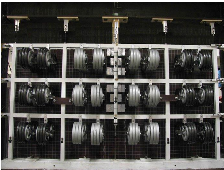
Fig. 4. Mechanism of static loading in Sagioglu's experiment (2012).
